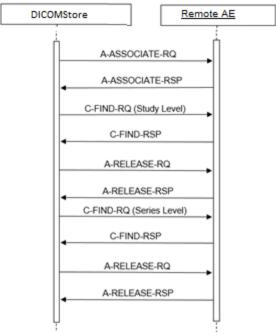
Figure 7: Data Flow Diagram – FIND as SCU
