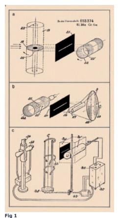
Optical image reconstruction from projections as patented by Gabriel Frank in 1938. Fig 1a. Projection of object (18) onto a cylindrical film
