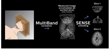
*MultiBand SENSE*: simultaneous acquisition of multiple slices to accelerate fMRI and dMRI in the brain. A phase shift between slices is used to facilitate SENSE unfolding for obtaining the individual images.
